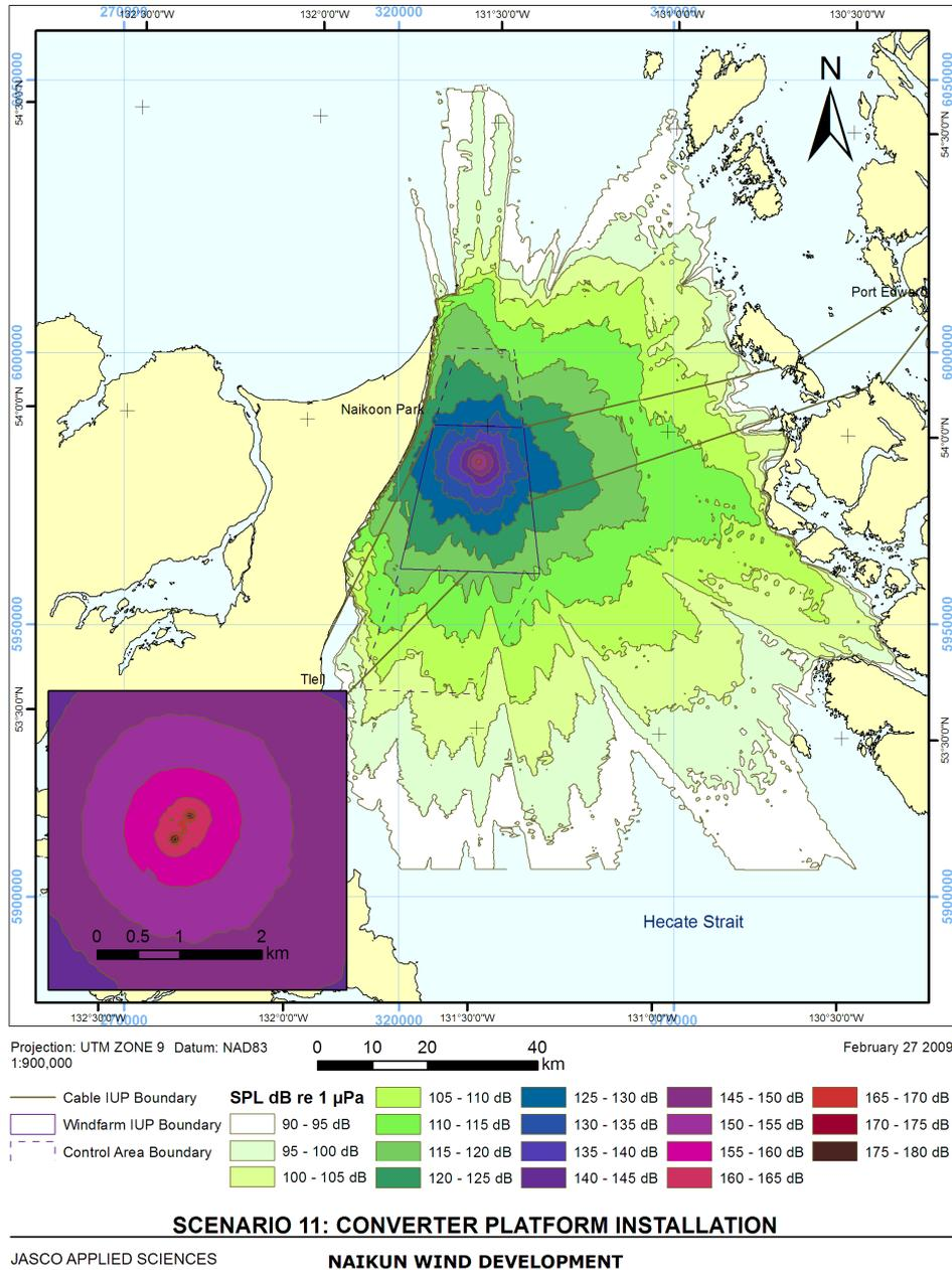
**Figure 9-14 Map Showing Modelled Noise Contours from the Installation of the Converter Platform using a Support Vessel and Supply Vessel on Standby, and Six Anchor Handling Tugs.**
