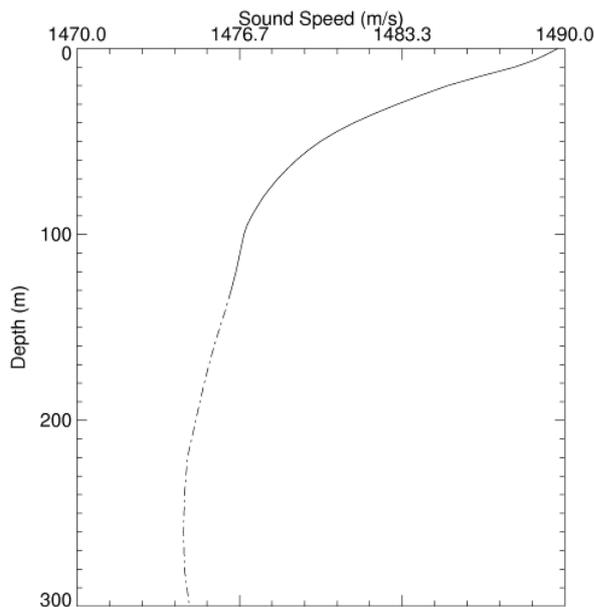
**Figure 8-3** Average Monthly Sound Speed in Water Plotted as a Function of Depth at the WFG for July.
