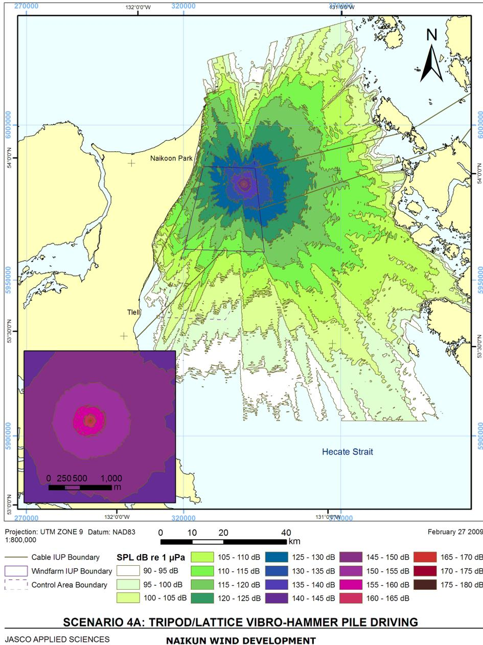
**Figure 9-6 Map Showing Modelled Noise Contours for Vibrohammering of a 2-3 m Diameter Steel Pile for the Tripod/Lattice Supports.**
