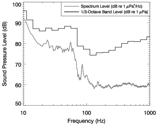
**Figure 8-1 Plot of a Typical Ambient Noise Power Spectrum (grey line) and the Corresponding 1/3-octave Band Levels (black line). Note that Frequency is Plotted on a Log Scale and so the 1/3-octave Bands are Wider at Higher Frequencies.**
