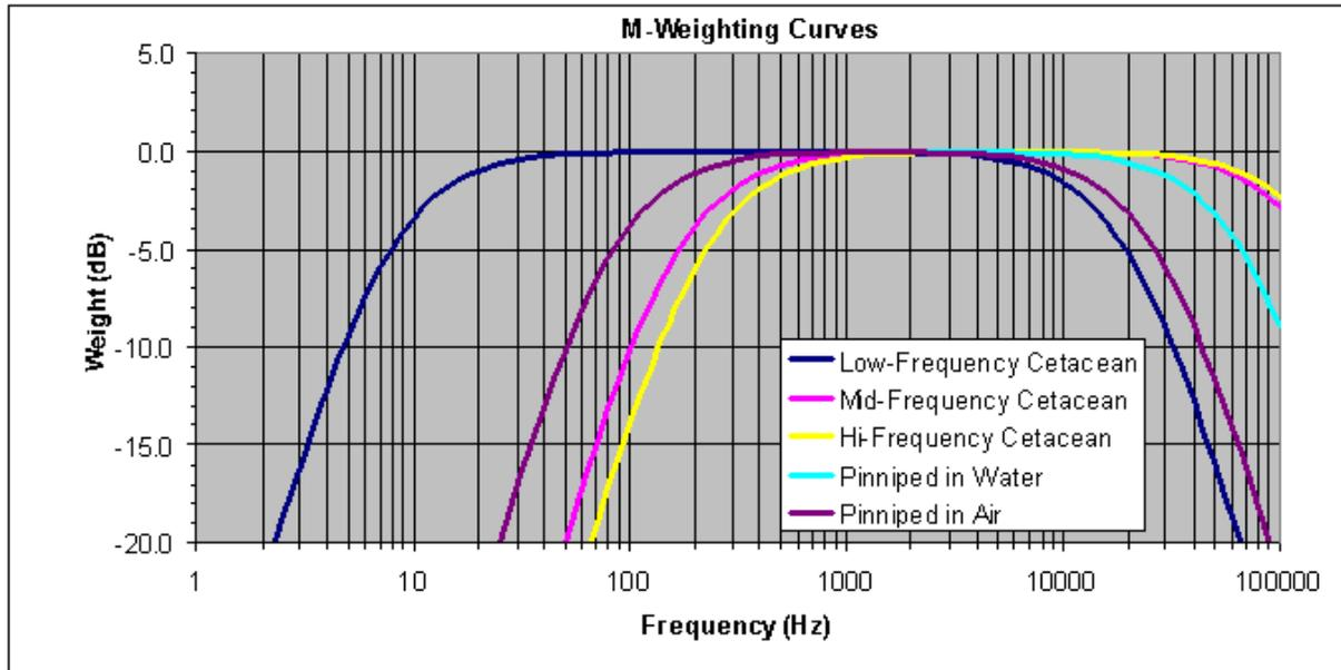
Figure 8-2 M-weighting curves for cetaceans and pinnipeds.
