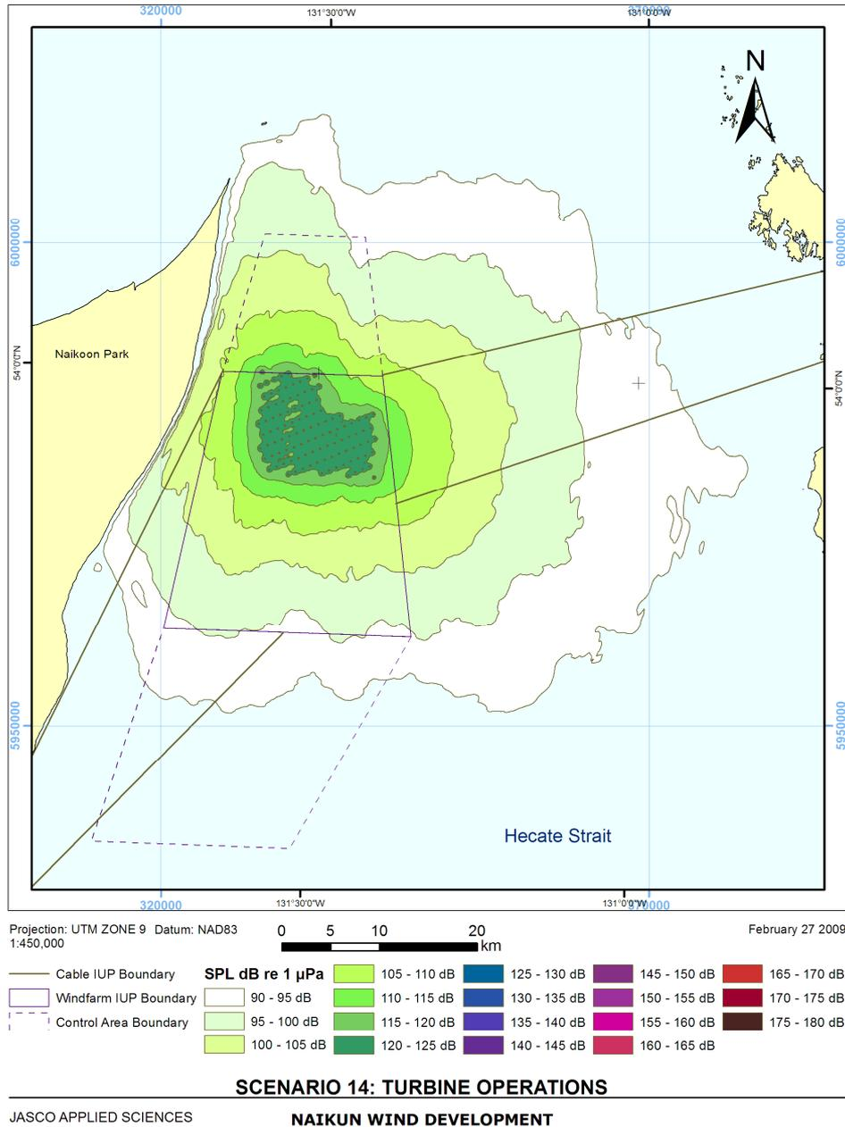
**Figure 9-17 Map Showing Modelled Noise Contours for Normal Operations of the WTGs (110 Siemens 3.6 MW turbines) at 8 m/s Wind Speed.**
