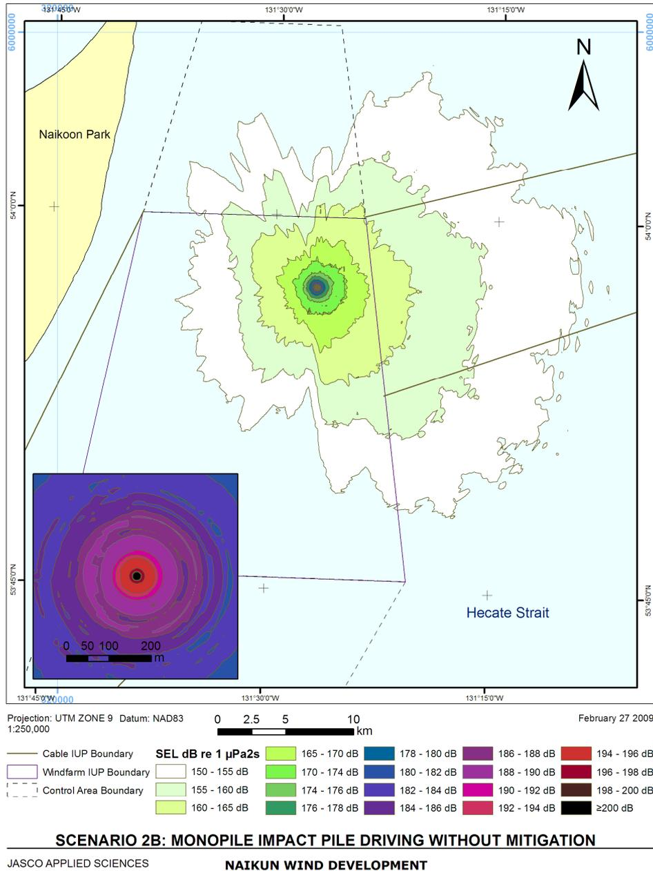
**Figure 9-3 Map Showing Modelled Noise Contours for Unmitigated Impact Hammer Pile Driving of a 4.5-5 m Diameter Steel Pile for the Monopile Supports (1200 kJ ram Energy).**
