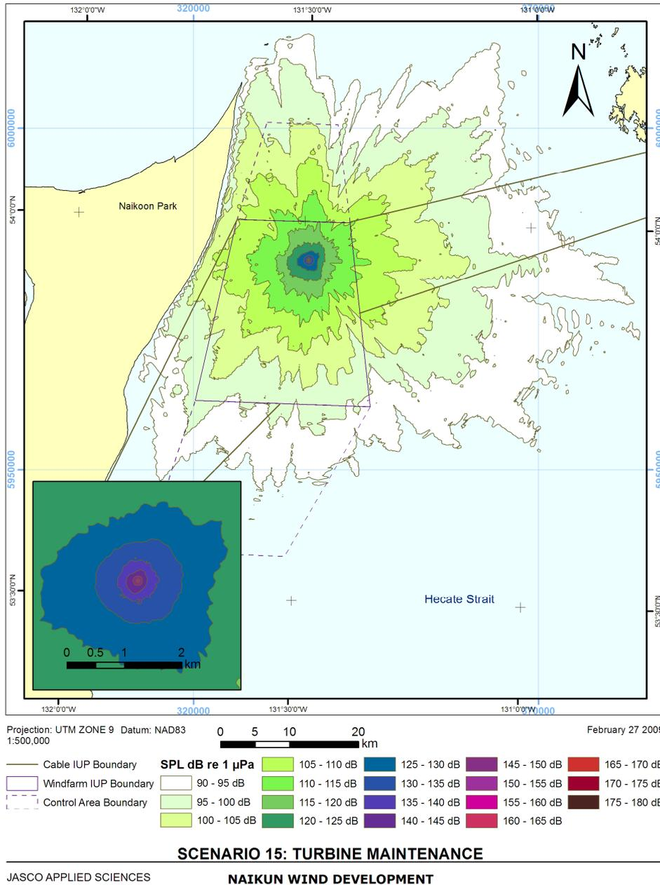
**Figure 9-18 Map Showing Modelled Noise Contours from Turbine Maintenance Activities using a Crew Vessel.**
