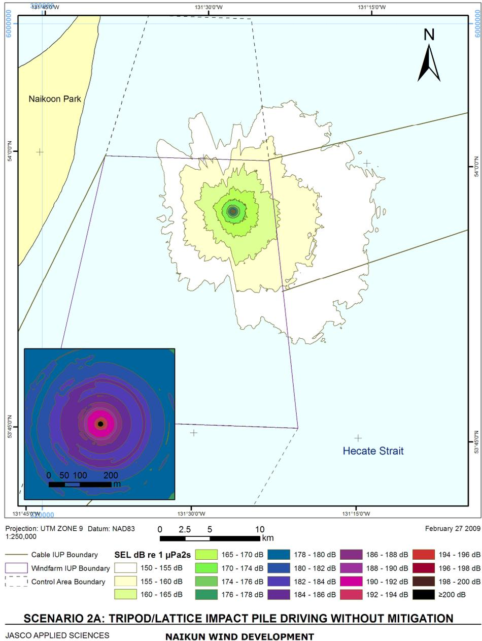
**Figure 9-2 Map Showing Modelled Noise Contours for Unmitigated Impact Hammer Pile Driving of a 2-3 m Diameter Steel Pile for the Tripod/Lattice Supports (550 kJ ram Energy).**
