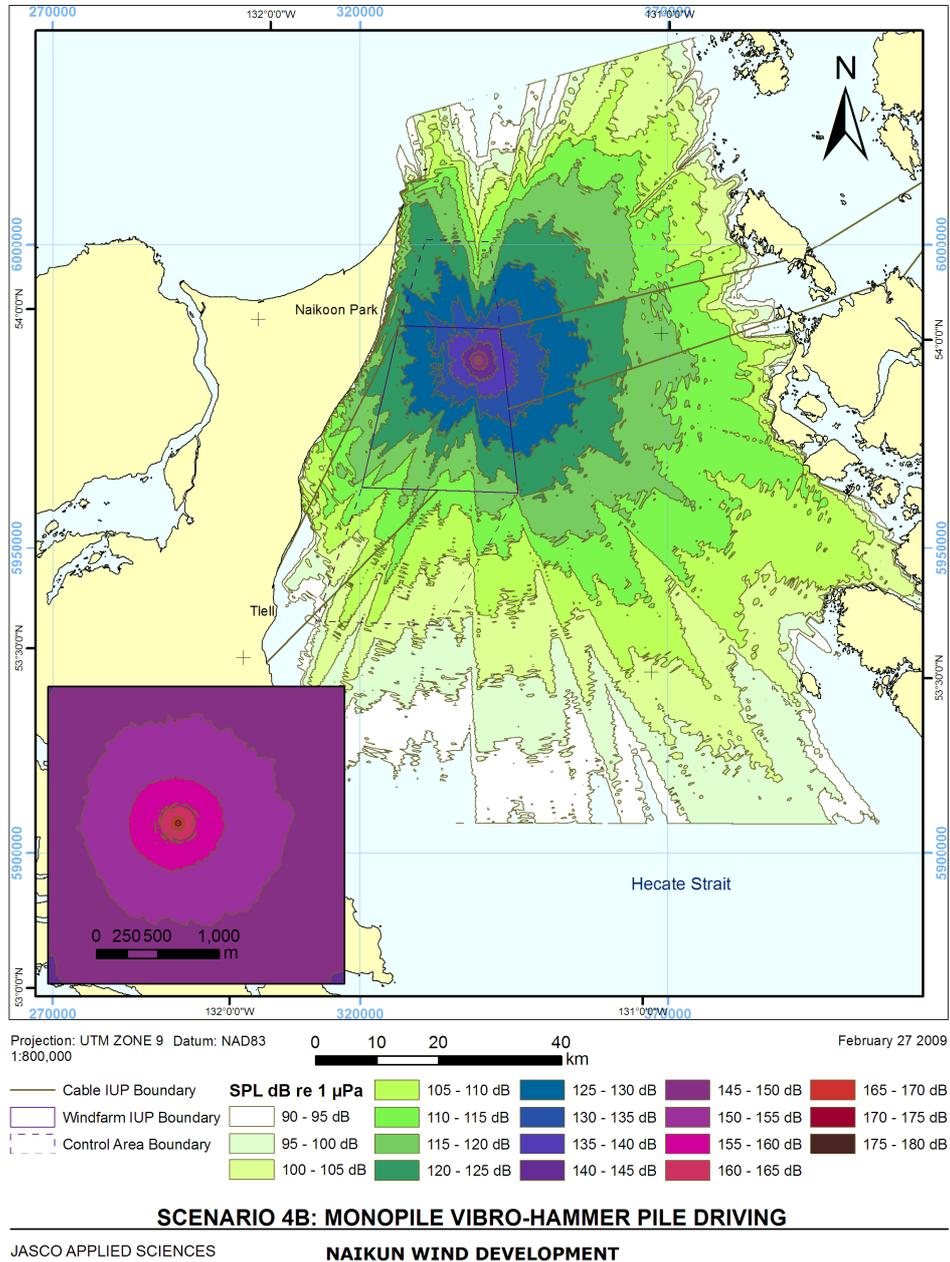
Figure 9-7 Map Showing Modelled Noise Contours for Vibrohammering of a 4.5-5 m Diameter Steel Pile for the Monopile Supports.
