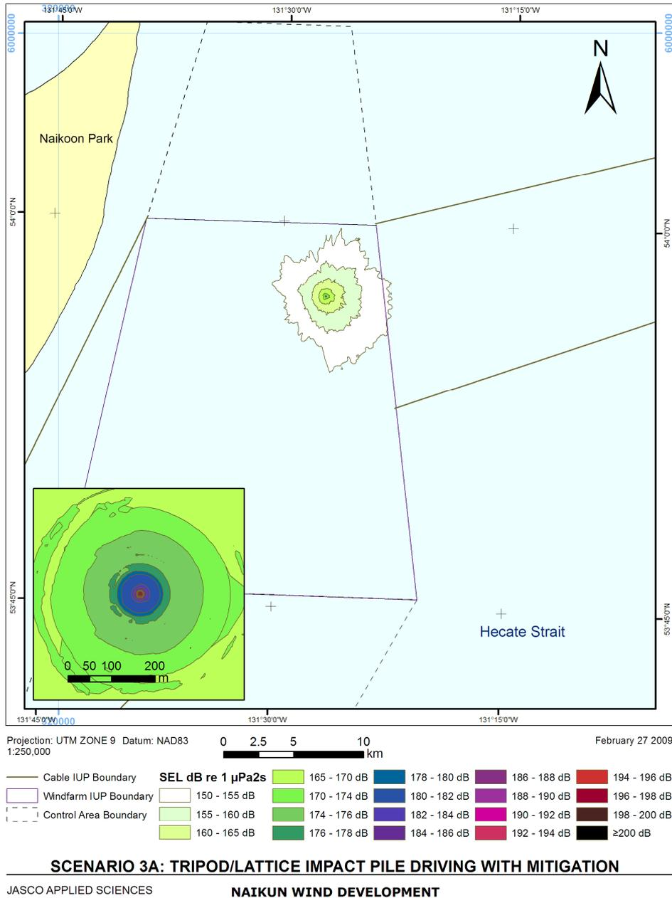
**Figure 9-4 Map Showing Modelled Noise Contours for Mitigated Impact Hammer Pile Driving of a 2-3 m Diameter Steel Pile for the Tripod/Lattice Supports (550 kJ ram Energy).**
