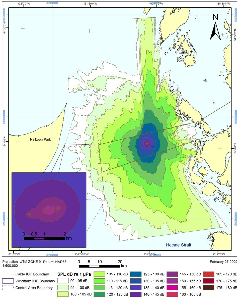
**SCENARIO 10: TRANSPORT OF CONVERTER PLATFORM TO WIND FARM GRID**
