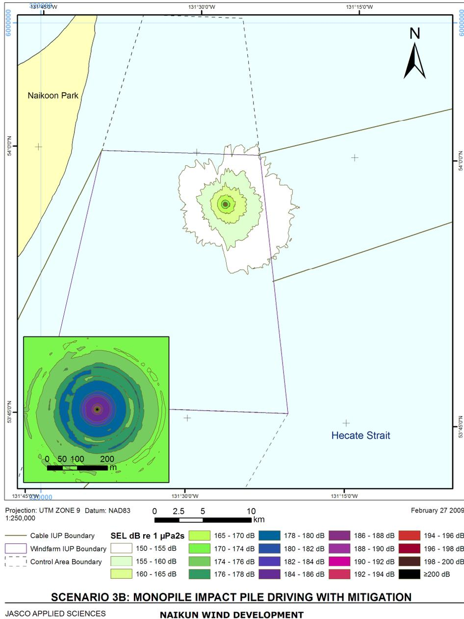
**Figure 9-5 Map Showing Modelled Noise Contours for Mitigated Impact Hammer Pile Driving of a 4.5-5 m Diameter Steel Pile for the Monopile Supports (1200 kJ ram Energy).**
